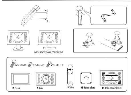
**Before you start:** Determine the position of the screen; Portrait or landscape and fix cell rubbers [H] position with tablet in the exact middle of the casing. (See manual - *Fixing the rubbers*) **Note:** Fitting the flat side of the tube [C] to the base plate [D] results in a straight tube (regular), mounting the diagonal side to the base plate results in an upward tube (variation).
